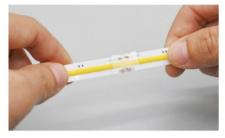
After complete the insert, also make sure both ends of led strip are tightly connected.
