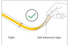
If the led strip needs to be torn up,please make sure that the self adhensive tape is torn with the led strip,otherwise the led strip will be damaged.
