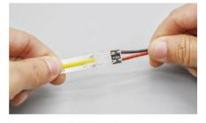
Insert one end of led strip and wire connector into both ends of the connection terminal respectively to ensure that the metal clip is on the same side as the metal solder pad of led strip.
